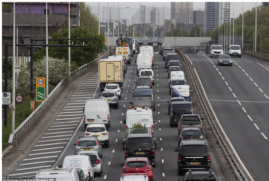
Figure: Directionally imbalanced traffic. Congested traffic in one direction and oppose direction having less traffic. 1
